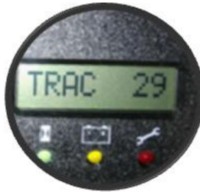
Figure 8-11 Curtis 840 meter fault display
